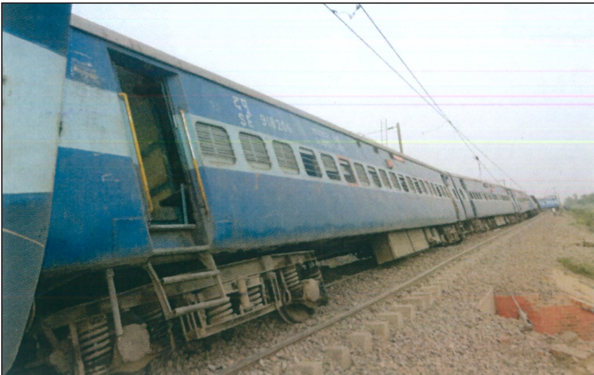
Derailed Coache S4 and Track with Deficient Shoulder Ballast
